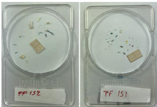
Figure III.11: Example of plastic particles extracted from sediments and seawater in Southwestern Madagascar. Particles are classified into two categories based on size: large particles (PF 152) and small particles (PF 151)
